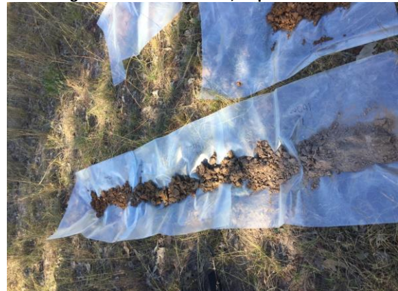
Figure 2: SS09 Soil Profile, Depth to 0.8 m
